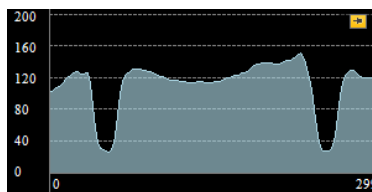
Appropriate inSmoothingStdDev - low noise, significant edges are preserved
