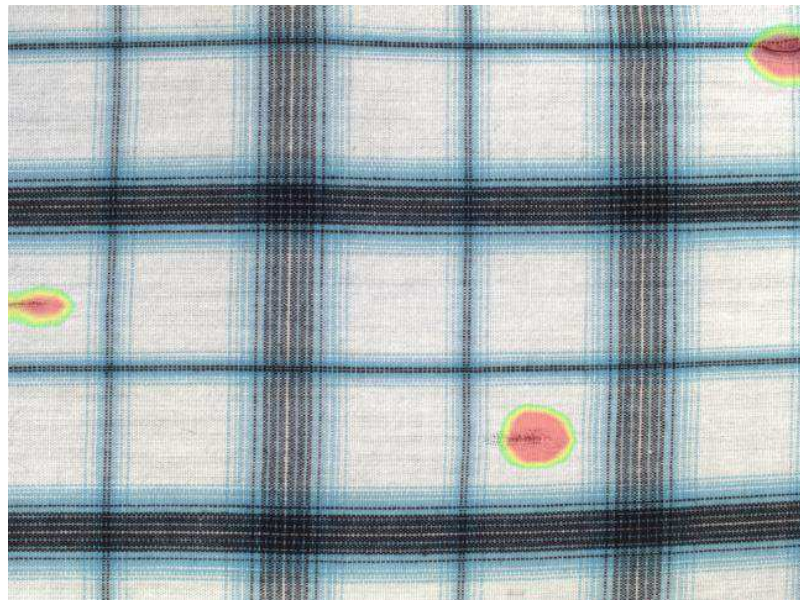
An example of textile defect detection using the DL_DetectAnomalies2 .
